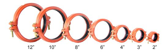
Grooved Fittings are a popular method of making pipe connections with larger diameter pipe in the Agricultural market. These fittings are compatible with grooved PVC pipe ranging in size from 2" through 12". Each cast iron fitting comes with a matching rubber seal and two bolts and nuts for a leak proof connection. Grooved fittings can be removed as needed and re-used with no gluing or cutting of pipe required.
